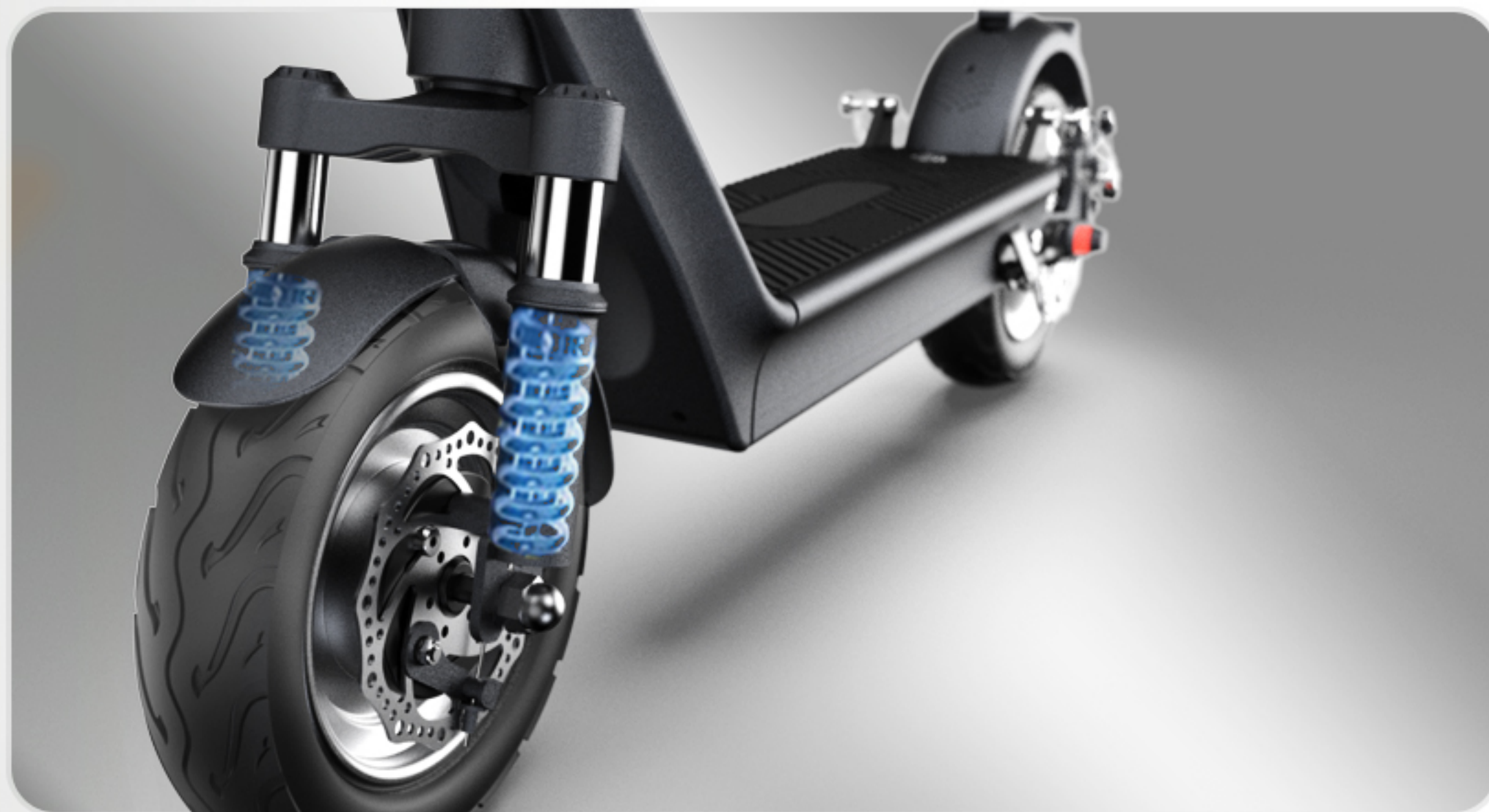
Front wheel dual-tube shock absorber structure
